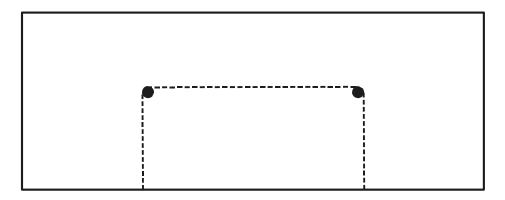
• All the inside corners should be rounded, with a minimum radius of 3/8", although at least 1/2" is recommended when possible. By eliminating the corners, you remove the weak points most susceptible to breakage.
