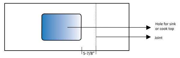
• The joint must not be positioned above the dishwasher or any other household appliance that radiates heat.
